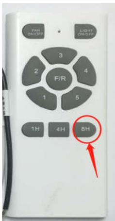
Note: To enter pairing mode, on the remote press and hold the 8H button for more than 5 seconds. You will hear 'Beep Beep' continuously indicating pairing mode.
