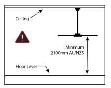
Provide adequate clearance from the floor. The lowest point on the fan blades must be at least 2.1m (7 feet) from floor level in Australia and at least 2.3m from floor level in the European Union and affiliated countries. Make sure that the chosen location of the fan will not allow the
